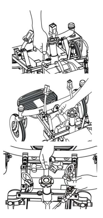
4. Let the cable pass through the hole of shroud.
