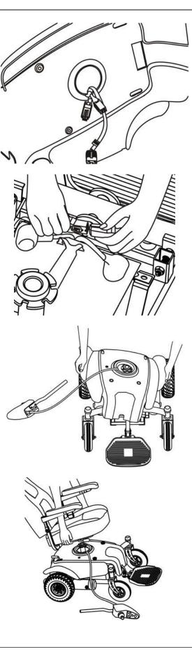
8. Swivel the seat and push down on the seat until it locks in place.
