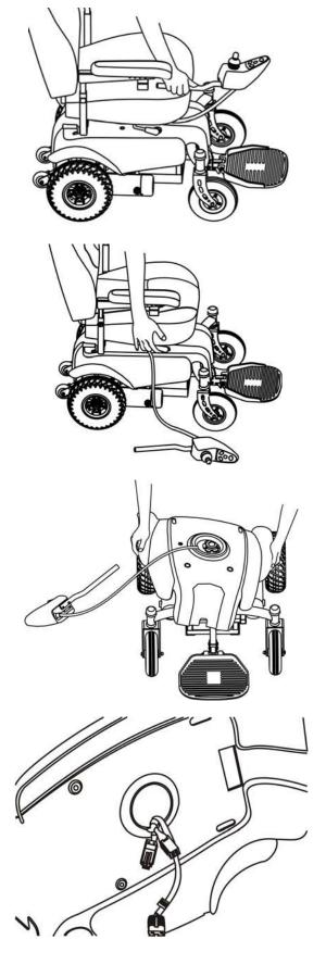
8. Disconnect both motor connectors with the main cable and the power cable.
